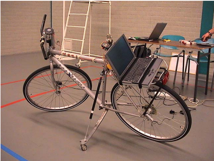
Fig. 2 Instrumented bicycle with all the measurement equipment installed. Sensors are present for measuring the roll rate, yaw rate, steering angle, and rear wheel rotation. Data are collected via a USB-connected data acquisition unit on the laptop computer, mounted on the rear rack
