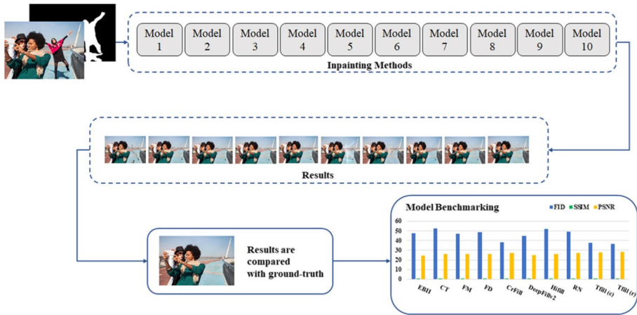
Fig. 6 The flowchart of the image de-photobombing benchmark in terms of FID [2], SSIM [3, 28], and PSNR [4, 5]
