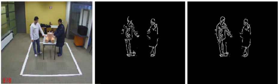
Fig. 3 Dynamic edge detector. Left : original image. Middle : dynamic edge by subtracting the edge in the background image from the edge of the current image. Right : our method
