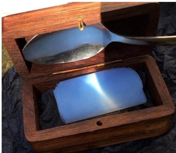
**Fig. 6** Experimenting with sunlight reflected on the concave mirror of a teaspoon. The sunlight ray concentration diagram we learned in physics is well visualized and documented as a three-dimensional sunlight hourglass. The half of the three-dimensional “X” has a bright white color and the other half has a golden hue because of the Rayleigh scattering phenomenon. A movie for this figure is also available in the Supplementary Material (Mov. S3). Photo and © MICHALOUS, 2020
