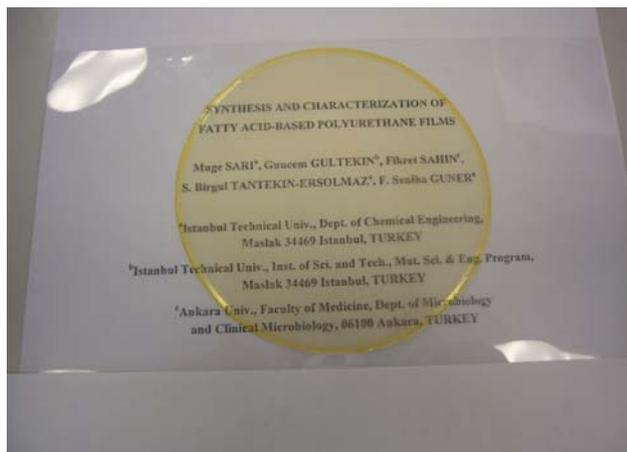
Fig. 11 Transparent dry polyurethane film
