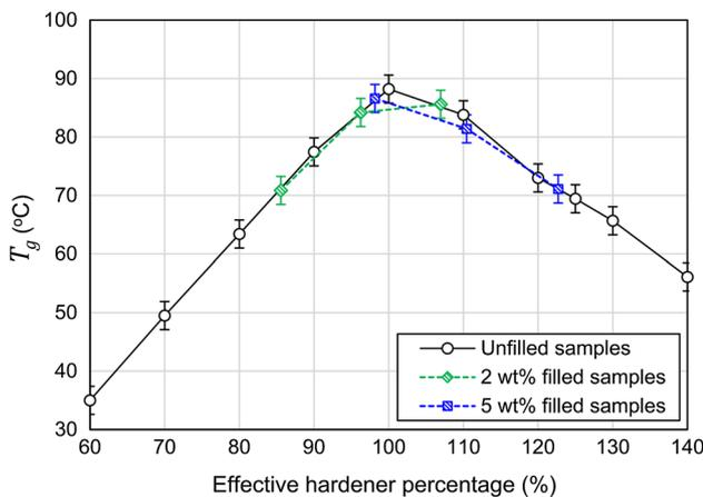
**Figure 2** *T<sub>g</sub>* of all samples as a function of effective hardener percentage.
