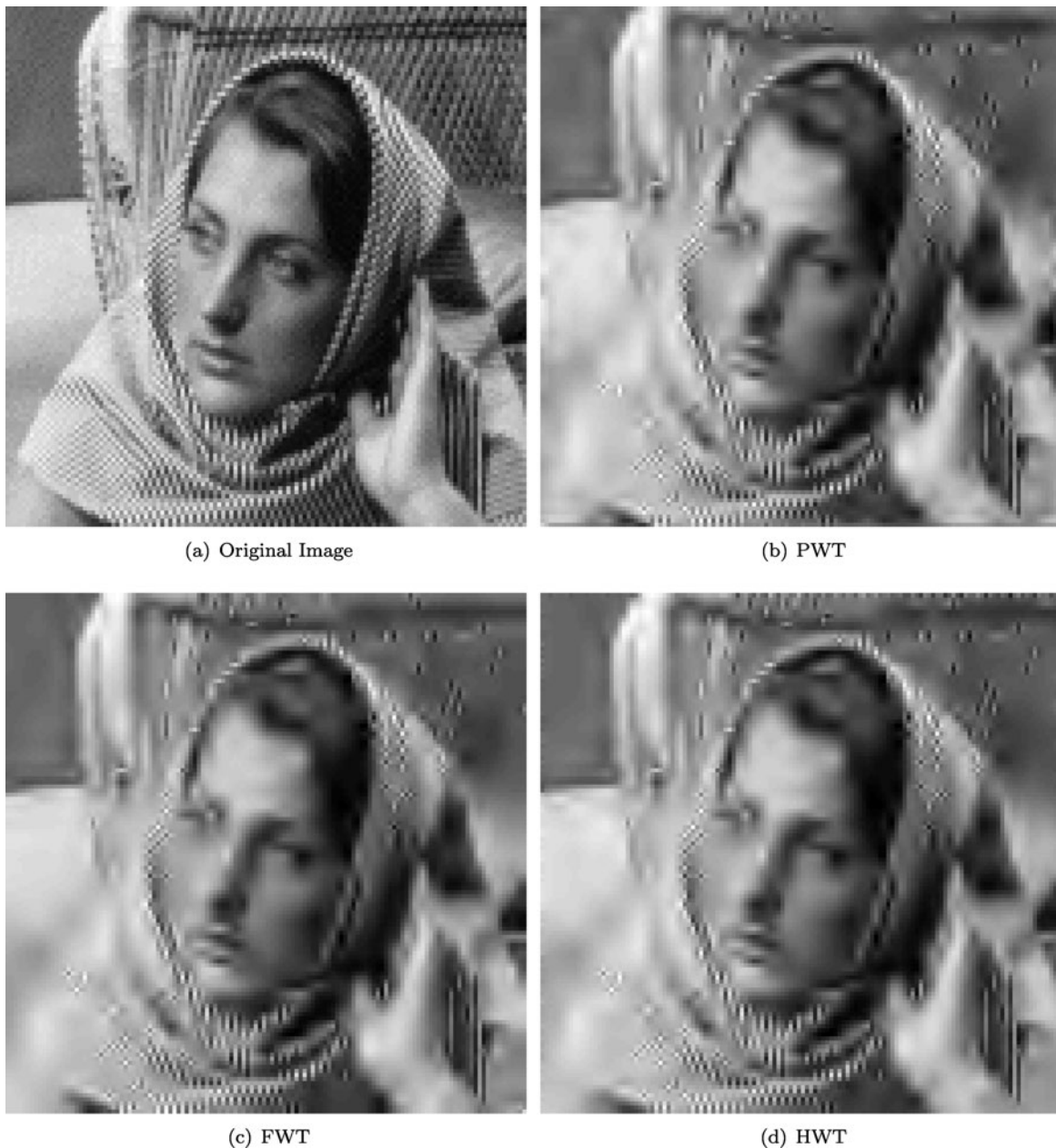
Fig. 10 Approximations of the Barbara face image using the top 5% coefficients when the depth of decomposition is seven. The PSNR values (in dB) of PWT, FWT, and HWT are 22.9962, 23.1476, and 23.2688, respectively
