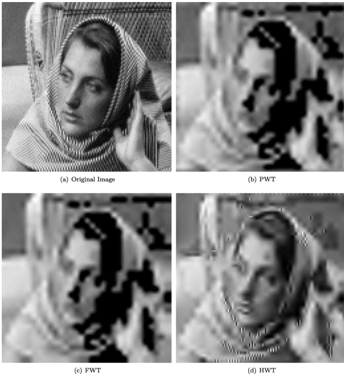
Fig. 8 Approximations of the Barbara face image using the top 5% coefficients when the depth of decomposition is two. The PSNR values (in dB) of PWT, FWT, and HWT are 17.6182, 17.5961, and 22.0776, respectively
