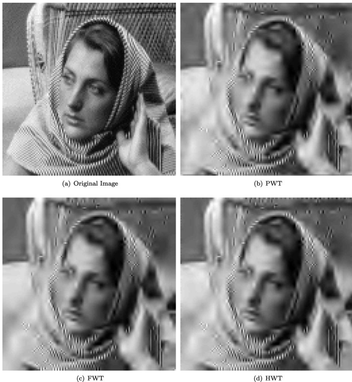
Fig. 9 Approximations of the Barbara face image using the top 5% coefficients when the depth of decomposition is four. The PSNR values (in dB) of PWT, FWT, and HWT are 22.9791, 23.1484, and 23.2651, respectively
