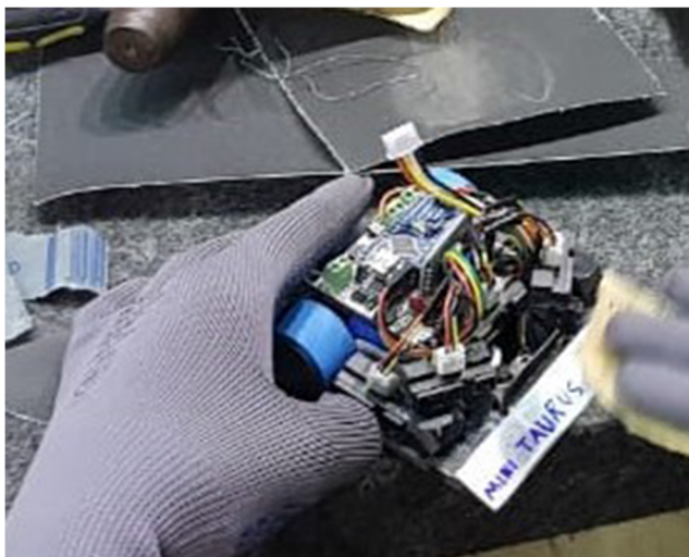
Fig. 2 Sumo robot developed by IFSP/RGT students being prepared for combat
