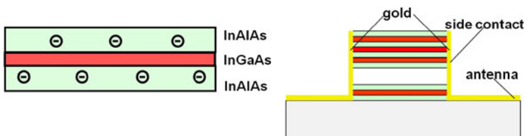
Fig. 6 Left: scheme for capturing of carriers from an InGaAs photoconductive film by InAlAs deep trapping centres. Right: improved mesa-structure with electrical side contacts for homogeneous fields and barrier-free current flow.
