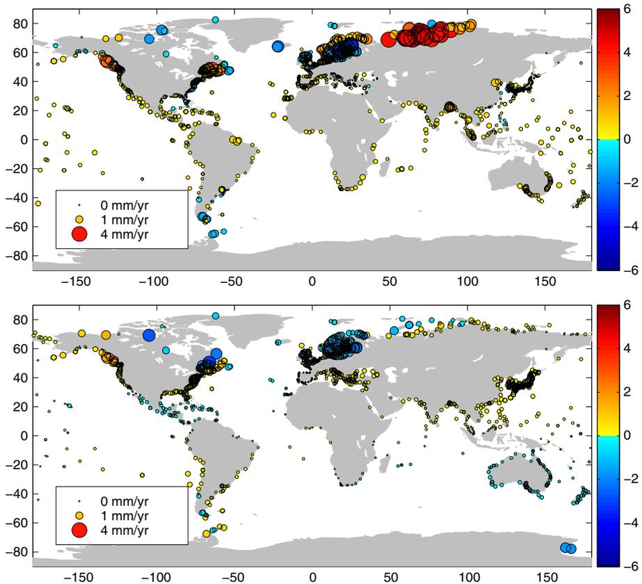
**Fig. 4** Maps of differences between GIA corrections from ICE 6G and ICE 4G (*top*) and ICE 6G and ICE 5G (*bottom*) at individual locations of tide gauges. *Color bar* in  $\text{mm year}^{-1}$  and *circle size* in  $\text{mm}$
