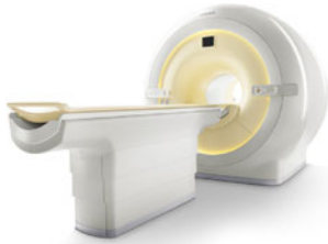
(a) Philips 3T Achieva system. The small opening (called the bore) is clearly visible. The casing around it holds the superconducting magnet as well as the liquid helium to cool it.
