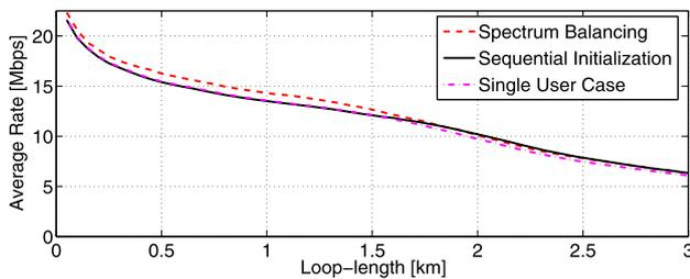
**Fig. 12** Average rate of 33 AN-enabled ADSL2+ lines under different performance evaluation techniques
