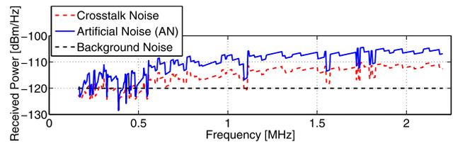
**Fig. 4** Relation between the crosstalk and artificial noise received on the shortest (800 m long) line for a margin of  $\gamma_u = 1$  dB,  $\forall u \in \mathcal{U}$ , in ADSL2+
