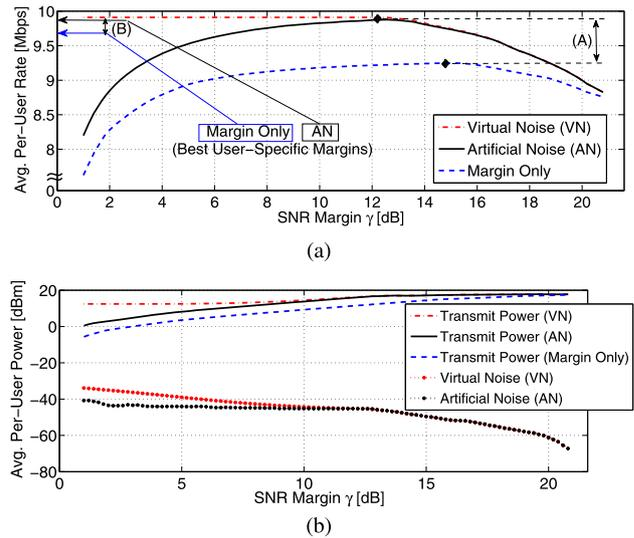
**Fig. 2** Dependency of the mean-rate (a) and transmit powers (b) of three stabilization techniques on the set SNR margin  $\gamma_u = \gamma, \forall u \in \mathcal{U}$  in ADSL2
