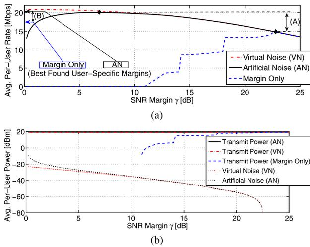
**Fig. 8** Average rates (a) and power levels (b) under three stabilization techniques and a worst-case crosstalk assumption in a distributed 3-user ADSL2+ scenario
