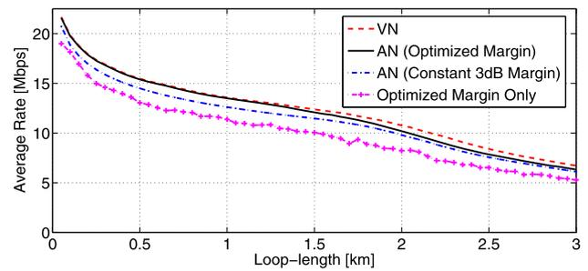
**Fig. 11** Average rate of 33 stabilized ADSL2+ lines under sequential initialization
