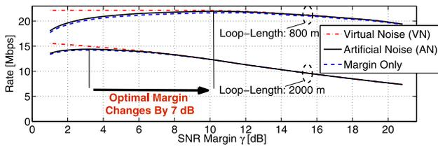
**Fig. 5** Dependency of the mean-rate on the single SNR margin  $\gamma_u = \gamma, \forall u \in \mathcal{U}$ , for three stabilization techniques in two collocated scenarios
