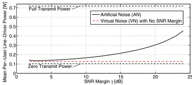
**Fig. 7** Dependency of the mean line-driver power consumption on the single SNR margin  $\gamma_u = \gamma$ ,  $\forall u \in \mathcal{U}$ , under AN compared to the optimal power under VN in a 33-user ADSL2+ scenario
