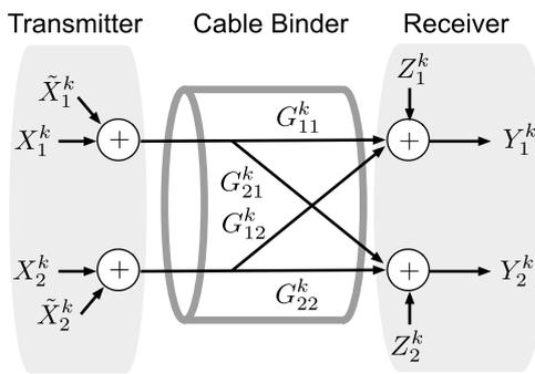
**Fig. 1** Downstream signal model for the DSL interference channel on subcarrier  $k$  for  $U = 2$  users highlighting the addition of the artificial noise  $\tilde{X}_u^k$  to the transmitted symbol  $X_u^k$ ,  $u \in \{1, 2\}$
