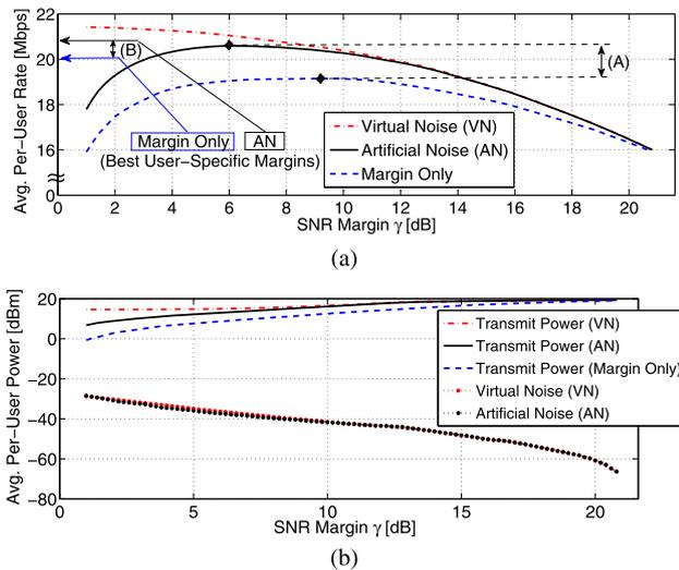
**Fig. 3** Dependency of the mean-rate (a) and transmit powers (b) of three stabilization techniques on the set SNR margin  $\gamma_u = \gamma, \forall u \in \mathcal{U}$  in ADSL2+
