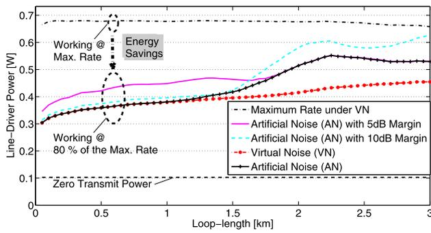
**Fig. 10** Line-driver power consumption of a single line under study operating at 80 % of the maximum (stable) achievable rate, under the three studied stabilization techniques and 30 collocated disturbers in ADSL2+
