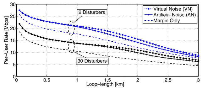
**Fig. 9** Rate under the three stabilization techniques in ADSL2+ for 2 and 30 collocated disturbers, respectively
