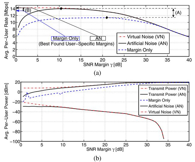
**Fig. 6** Dependency of the mean-rate (a) and transmit powers (b) of three stabilization techniques on the set SNR margin  $\gamma_u = \gamma, \forall u \in \mathcal{U}$  in ADSL2+ with 33 lines
