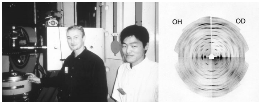
Fig. 2 The recording of hydrogenated and deuterated high-resolution neutron fiber diffraction patterns of I\beta cellulose by Paul Langan and Yoshiharu Nishiyama at ILL, Grenoble in 2002
