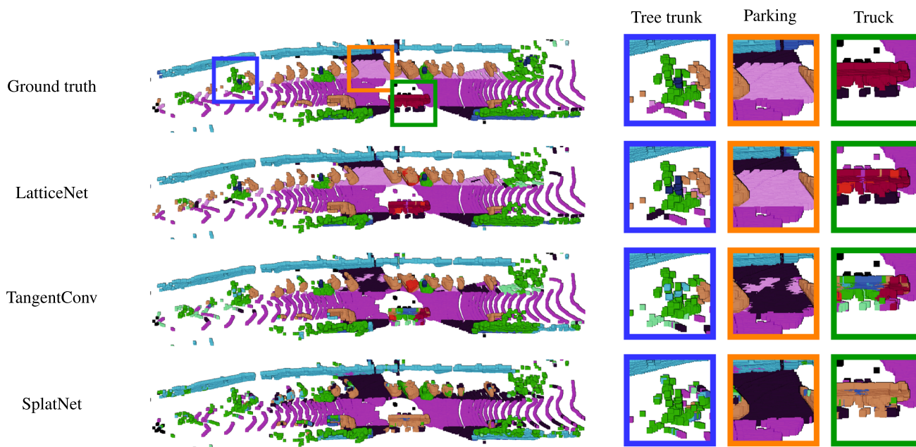
Fig. 13 SemanticKITTI results. We compare the prediction from our LatticeNet with the results from TangentConv (Tatarchenko et al. 2018) and SplatNet (Su et al. 2018). We can observe that our approach can better learn small objects like tree trunks, despite their relatively small
