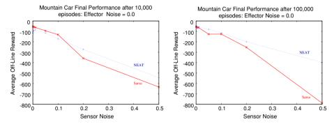
Fig. 11 A comparison of the average reward of the policies discovered by NEAT and Sarsa after 10,000 episodes (*left*) or 100,000 episodes (*right*) in mountain car variations with different levels of sensor noise
