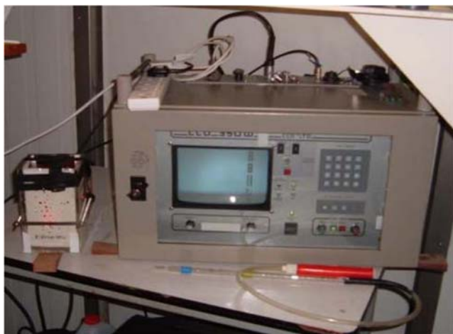
Fig. 1 Image of the LabSFLOC instrumentation: settling column (left), camera control unit (right) and modified floc extraction pipette (front right)
