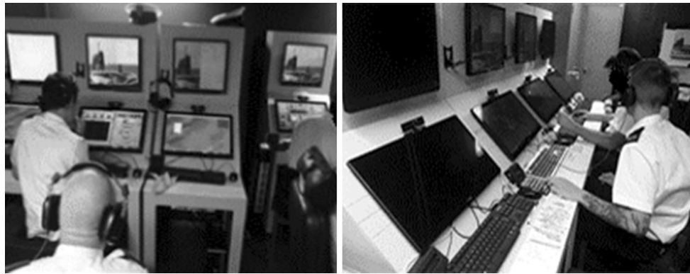
Fig. 1 The ComTET submarine control room simulator, with sound room on the left and picture room on the right
