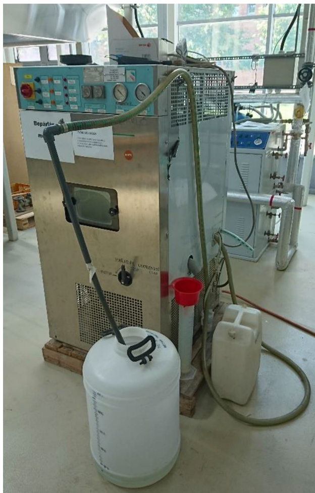
Fig. 3 Aquamove™ EVALED™ R-150 v3 pilot heat pump scraped vacuum evaporator (Veolia Water 2017)
