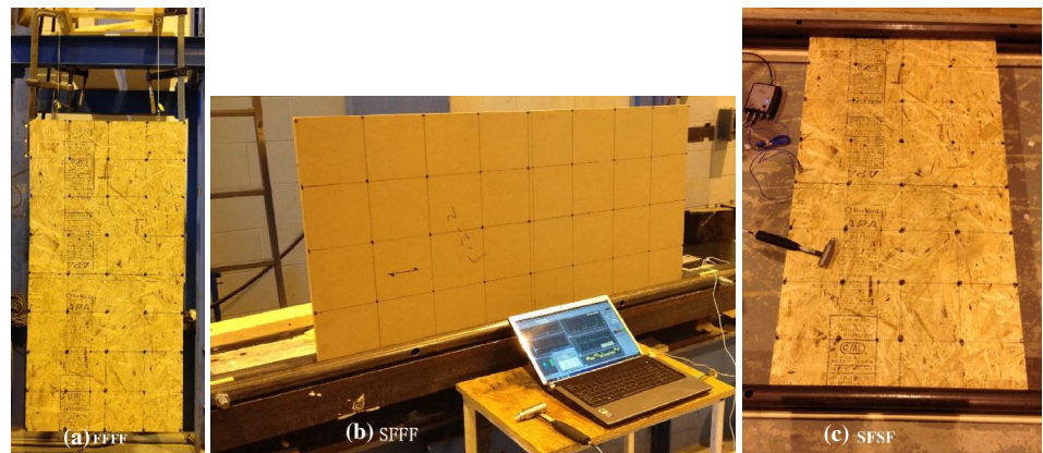
Fig. 4 Test setups for modal tests under different boundary conditions ( solid circle refers to the location of accelerometer and blank circle (I1–3) refers to the impact location)
