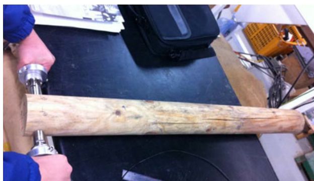
Fig. 4 Test set-up in order to obtain the ultrasonic waveforms
