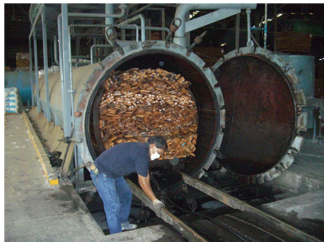
Fig. 3. Vacuum-pressure process for treatment of sawn rubberwood 21
