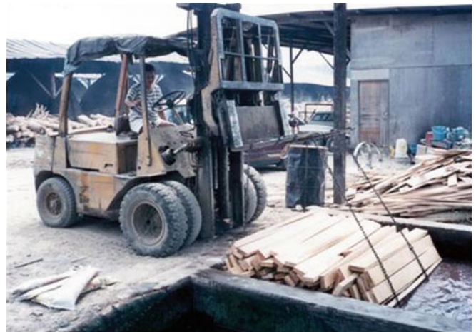
Fig. 2. Dipping of freshly sawn rubberwood in preservative mixture 21
