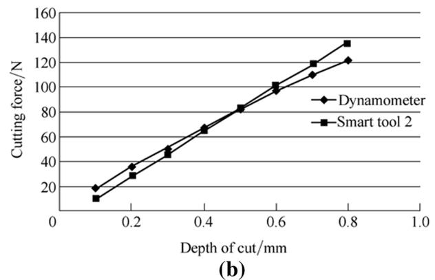
**Figure 5** Cutting force measurement with **a** smart tool 1, **b** smart tool 2, and calibration against Kistler dynamometer
