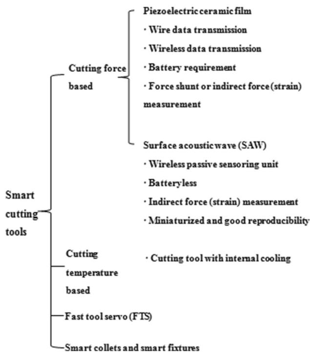
Figure 1 Family schematic of smart cutting tools
