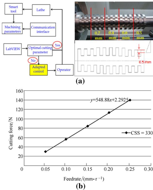
**Figure 18** **a** Adaptive control loop and adaptive smart machining trails on a CNC machine; **b** the relationship between the federate and cutting force
