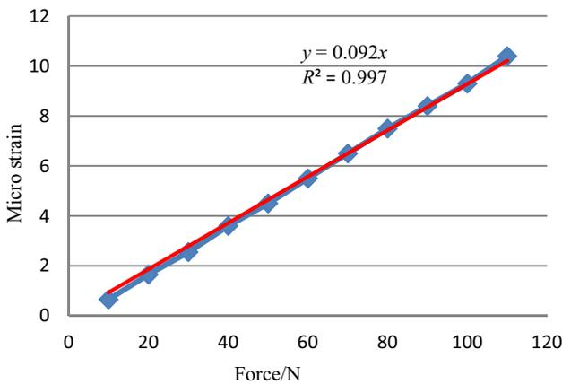
**Figure 11** Correlation between static force and strain output
