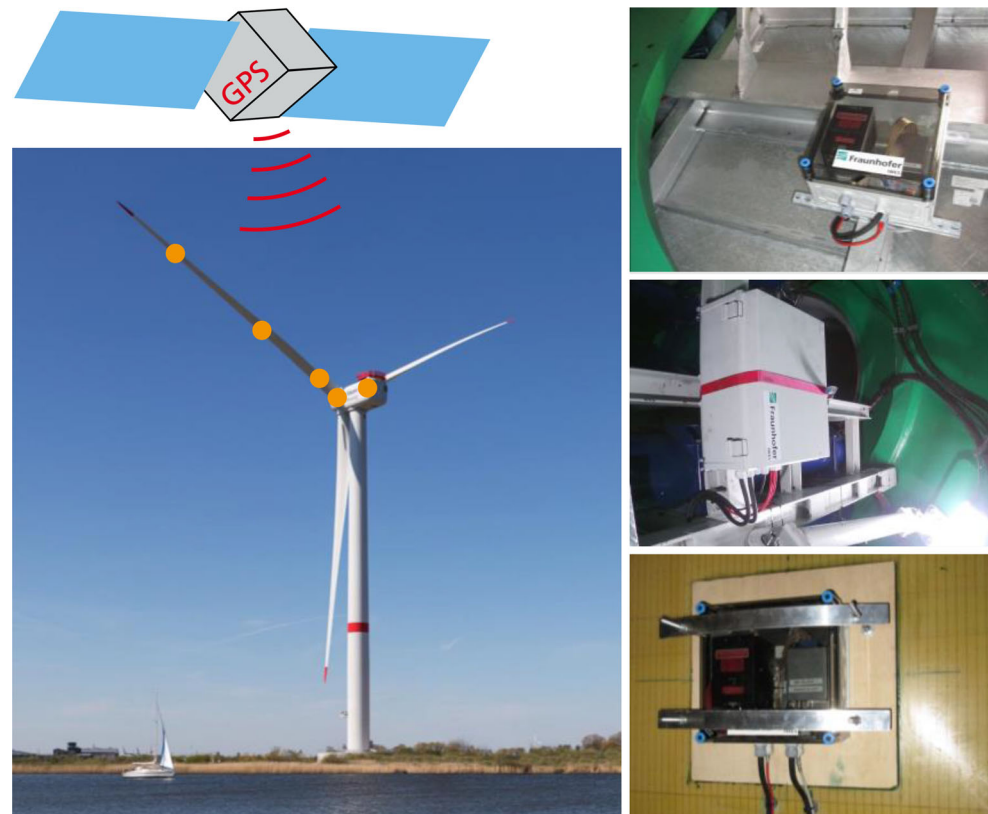
Fig. 2 Mounting locations on the Adwen AD 8–180 WEC (left) and pictures of mounted IMUs in nacelle and blade and PLC in the hub (right)
