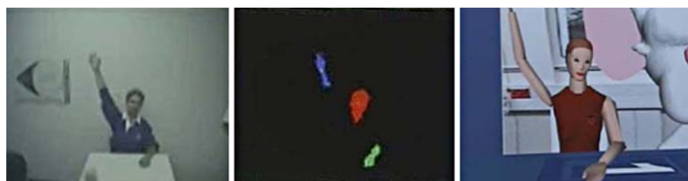
Fig. 3 Remote participant, making some gesture, the gesture recognition, and the representation within the VMR, as seen through the eyes of one of the other participants
