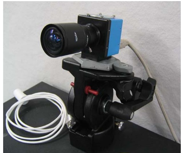
Fig. 5 Industrial Firewire camera
