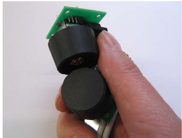
Fig. 7 Assembly of rotary encoder wheels to manipulate menus and variables
