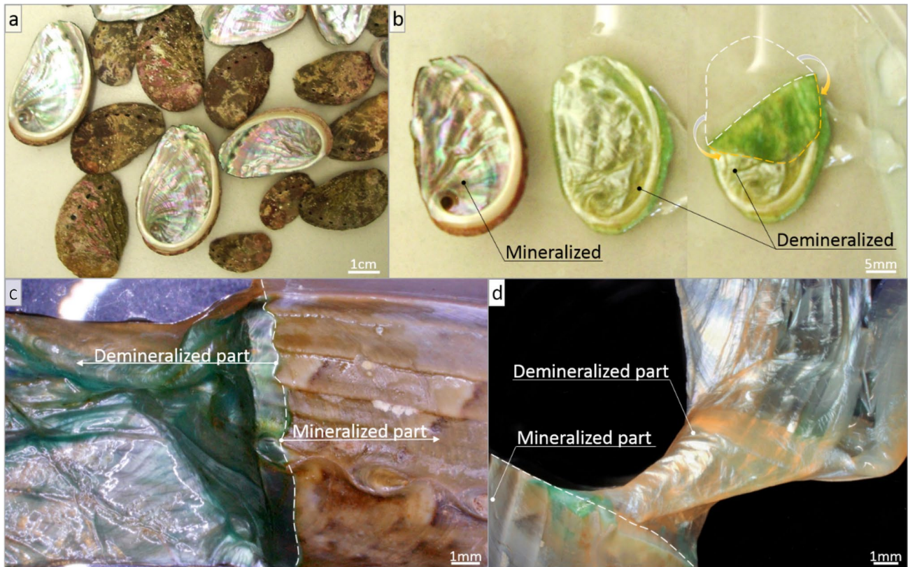
Fig. 8 Shells of H. tuberculata (a) constitute a massive waste of the marine processing industry. They can be effectively demineralized with Osteosoft solution at 37 °C during 3–5 days with the aim
