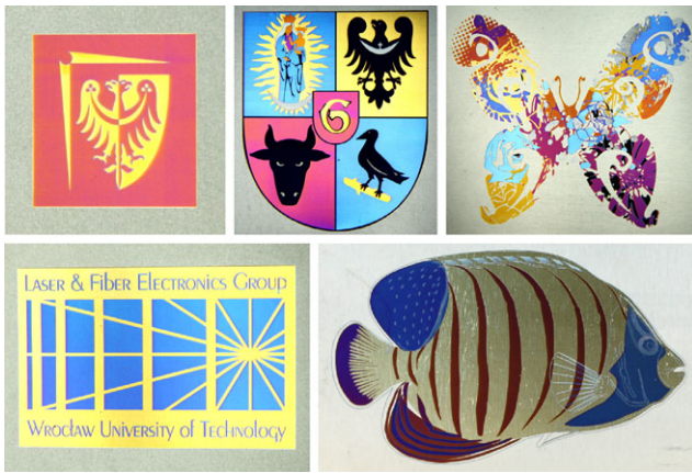
Fig. 14 Examples of color laser marking on titanium. Trademarks and trade names are the exclusive property of their respective owners. They are used only to demonstrate the possibilities of laser color marking
