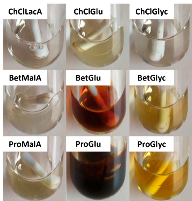
Fig. 2 Extracts obtained after extraction by MAE at 130 °C for 10 min using different NADES as extracting solvents. Reproduced with permission from [32]
