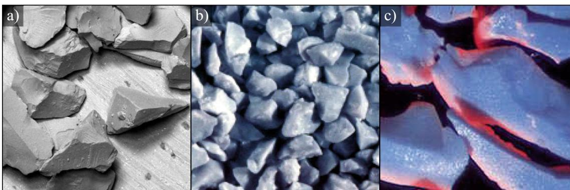
**Fig. 7** View of the microcrystalline sintered corundum grains: **a** SG<sup>TM</sup> grains—magnification  $\times 100$ ; **b** Cubitron 321<sup>TM</sup>—magnification  $\times 50$  [16]; **c** Sapphire Blue<sup>TM</sup> grains—magnification approx.  $\times 500$  [21]
