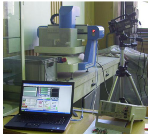
Fig. 6 A general view of the test bench (control unit+mini-grinder SIC330 CNC+digital power analyser DW6090+thermal camera FLIR SC620)
