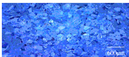
Fig. 4 The structure of a grinding wheel made of microcrystalline sintered corundum, abrasant content 5CB
