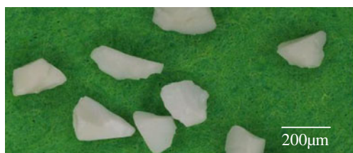
Fig. 2 A general view of abrasant grains made of microcrystalline sintered corundum CB, grain number 60
