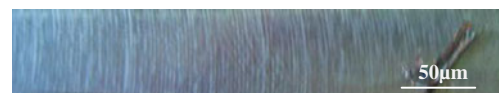
Fig. 19 A view of the machined surface, with a sticking chip removed from the active grinding wheel's surface
