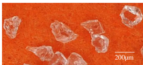
Fig. 1 A general view of abrasant grains made of white noble electrocorundum 99A, grain number 60
