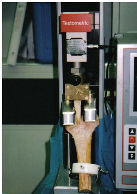
Fig. 1 Tensile testing set-up, showing adjustable femoral condyles
