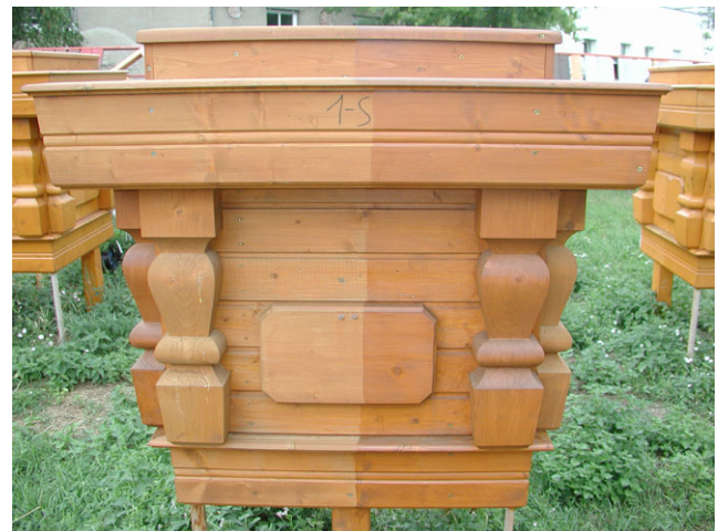
Fig. 1 Front view of balcony construction, side exposed to south; left side : original coating; right side : maintenance coating (applied after 18 months of exposure)
