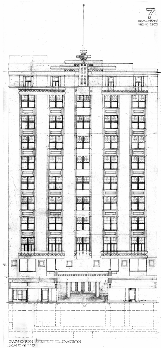
Fig. 4. Permit Drawing 7 (dated 1921.10.29): Swanston Street elevation showing the unbuilt finial and central tribunes. Melbourne University Architectural Collection, State Library of Victoria. Image processing by Keith Lo Bue
