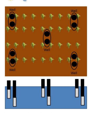
Fig. 7 Schematic diagram of an in-field groundwater monitoring study
