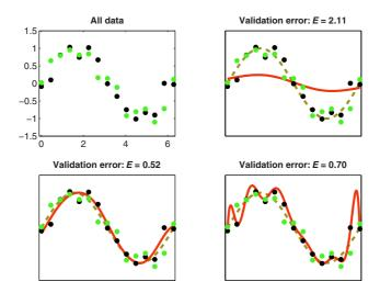
**Fig. 2.** Function estimates (solid line) and validation error for three different values of regularisation hyperparameter  $\lambda$  (the true function is shown dashed). The training data is plotted in black, and the validation set in green (gray)
