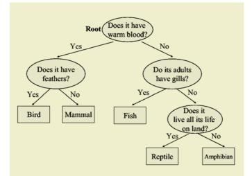
**Fig. 4.** An example a decision tree. Classification of a new test point is achieved by moving from top to bottom along the branches of the tree, starting from the root node, until a terminal node (square) is reached
