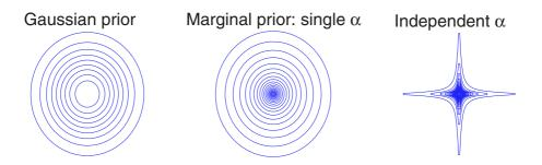
Fig. 8. Contour plots of Gaussian and Student-t prior distributions over two parameters. While the marginal prior  $p(w_1, w_2)$  for the 'single' hyperparameter model of Section 2 has a much sharper peak than the Gaussian at zero, it can be seen that it is not sparse unlike the multiple 'independent' hyperparameter prior, which as well as having a sharp peak at zero, places most of its probability mass along axial ridges where the magnitude of one of the two parameters is small
