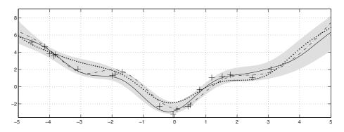
**Fig. 2.** Three functions drawn at random from the posterior, given 20 training data points, the  $\mathcal{GP}$  as specified in Eq. (3) and a noise level of  $\sigma_n = 0.7$ . The shaded area gives the 95% confidence region. Compare with Figure 1 and note that the uncertainty goes down close to the observations
