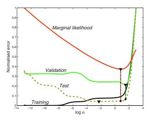
Fig. 5. Plots of the training, validation and test errors of the model as shown in Figure 3 (with the horizontal scale adjusted appropriately to convert from  $\lambda$  to  $\alpha$ ) along with the negative log marginal likelihood evaluated on the training data alone for that same model. The values of  $\alpha$  and test error achieved by the model with highest marginal likelihood (smallest negative log) are indicated
