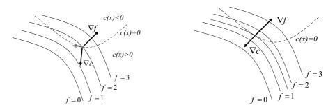
Fig. 1. At the constrained optimum, the gradient of the constraint must be parallel to that of the function
