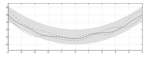
Fig. 1. Function values from three functions drawn at random from a GP as specified in Eq. (2). The dots are the values generated from Eq. (4), the two other curves have (less correctly) been drawn by connecting sampled points. The function values suggest a smooth underlying function; this is in fact a property of GPs with the squared exponential covariance function. The shaded grey area represent the 95% confidence intervals
