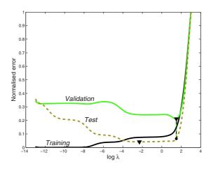
Fig. 3. Plots of error computed on the separate 15-example training and validation sets, along with 'test' error measured on a third noise-free set. The minimum test and validation errors are marked with a triangle, and the intersection of the best  $\lambda$  computed via validation is shown
