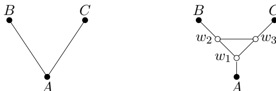
Figure 8. Triangle gadget. The interaction pattern on the left is simulated by the interaction pattern on the right by first applying the subdivision gadget to edges AB and AC , and then applying the fork gadget to qudit A .
