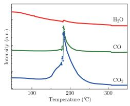
Fig. 2 The Mass Spectra of  $H_2O$ , CO, and  $CO_2$  as a function of temperature with a heating rate of  $10^{\circ}C/min$ , respectively.
