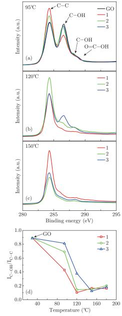
Fig. 3 C 1s XPS results of GO reduced under different temperature: 95°C (a), 120°C (b), and 150°C (c); the intensity ratio of C-OH and C-C peaks as a function of temperature (d). The samples were placed 1: under deionized water in a sealed Teflon autoclave (hydrothermal method), 2: under vacuum in a sealed quartz tube (with the pressure of several Pascal), and 3: in the air directly.
