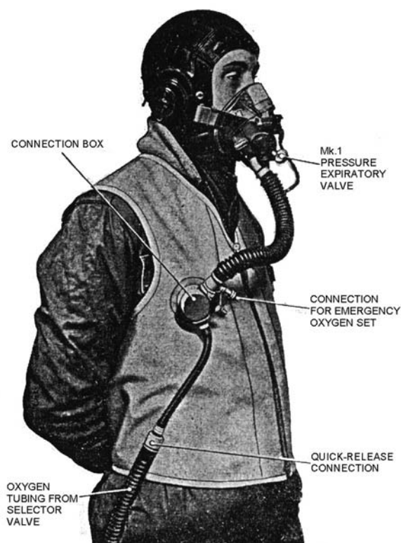
FIGURE Early pressure breathing mask and waistcoat. Picture sourced from a previously "RESTRICTED" September 1952 British Admiralty/Air Ministry publication, stored in the Royal Air Force Museum, Hendon, London NW9 5LL and identified as 'Air Publication 1275G, Vol 1, Sect. 3, Chapter 8: pressure breathing equipment'. Annotations reprinted, with the wording unchanged. ©British Crown Copyright/MOD. Reproduced with the permission of the Controller of Her Majesty's Stationery Office.
