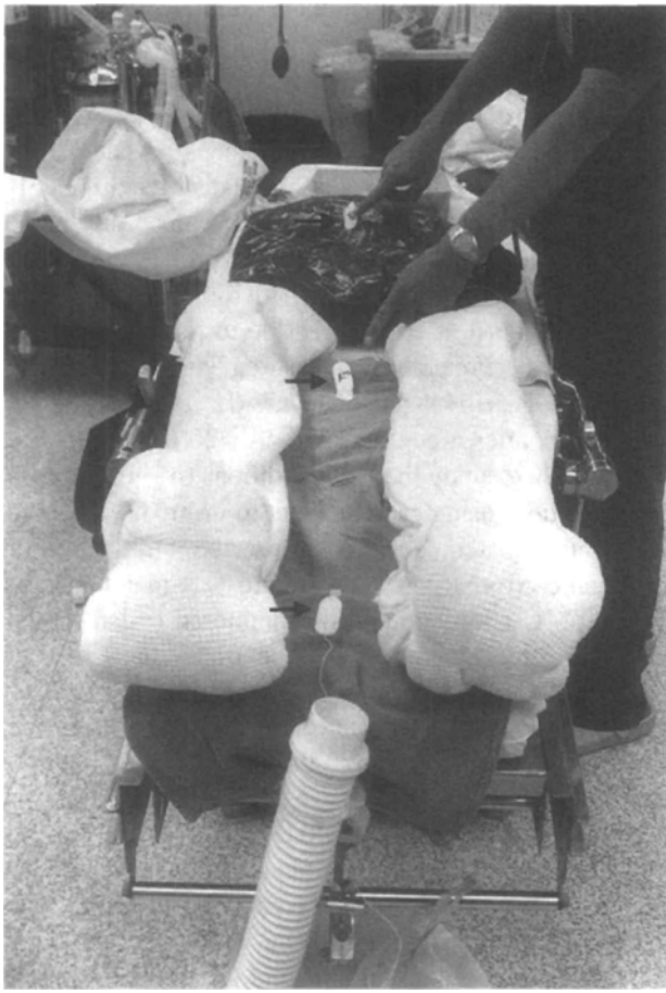
FIGURE 1 Blankets are in position to simulate the geometry of a human body within the full body field, shown before the test blanket is applied. The locations of temperature probes are indicated by arrows. The heating unit is seen introduced from the foot end in this and subsequent photographs.
