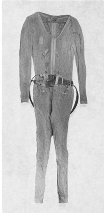
Fig. 3. Apollo liquid cooled garment (LCG). Cooled water is distributed by manifolds at the waist, flows in small tubes through the garment, and returns for collection again at the waist. (Photograph courtesy of National Aeronautics and Space Administration.)
