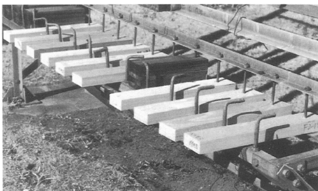
Fig. 1. Steel rack for outdoor exposure test
