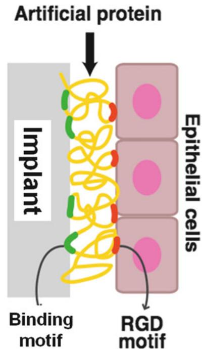
**Fig. 3.11** Schematic representation of an artificial protein intermediating between the surface of titanium and cells. Artificial proteins are shown as yellow containing Ti binding motif (TBP: *green*) and a cell binding motif (RGD: *red*) [22]
