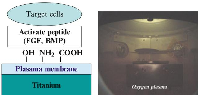
Fig. 3.13 Plasma treatment was performed using the VEP-1000 system (right) and schematic image shows the attachment of cells on the plasma treatment titanium surface (left)
