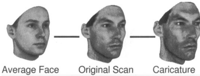
Figure 4: The comparison the 3D model of an individual face to the average face allows for exaggerating the characteristics of that face. After establishing correspondence between all example faces (200), the average face can be computed. Here a caricature of the face was obtained by increasing the difference of its shape and of texture vectors to the average face by a factor of two.
