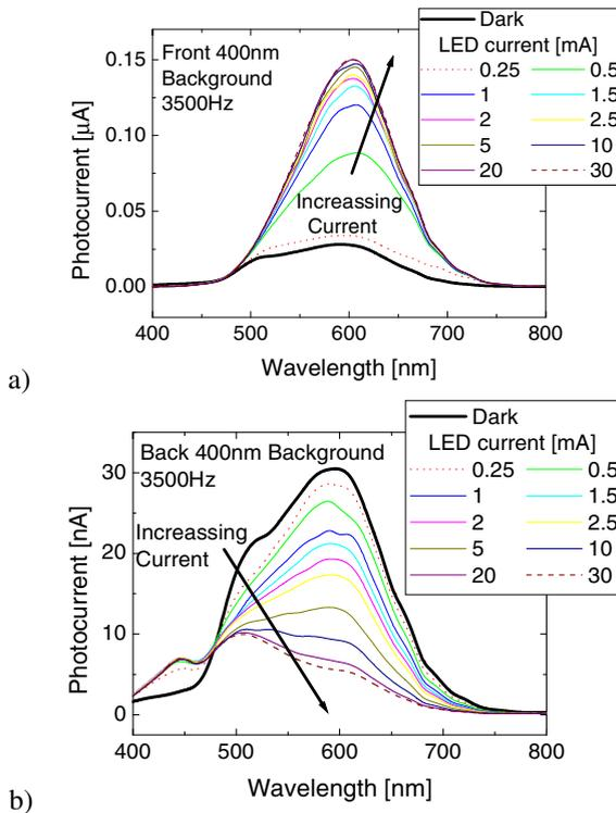
Fig. 2. Photocurrent with a) front and b) back lighting of the background
