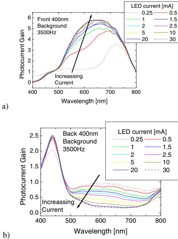
**Fig. 3.** Photocurrent gain when background light is at the a) front and b) back side of the device
