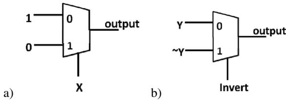
**Fig. 6.** A multiplexer used as an invert function
