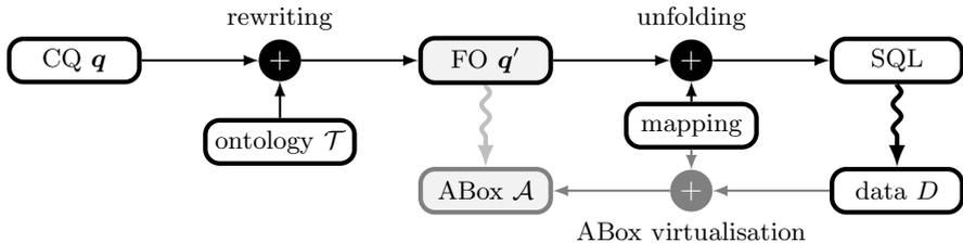
The user is given an OWL2 QL ontology  $\mathcal{T}$  and can formulate CQs  $q(\mathbf{x})$  in the signature of  $\mathcal{T}$ . The system rewrites  $q$  and  $\mathcal{T}$  into an FO-query  $q'(\mathbf{x})$ , called a *rewriting* of  $q$  and  $\mathcal{T}$ , such that  $(\mathcal{T}, \mathcal{A}) \models q(\mathbf{a})$  iff  $\mathcal{A} \models q'(\mathbf{a})$ , for any set  $\mathcal{A}$  of ground atoms (called an ABox) in the signature of  $\mathcal{T}$  and any tuple  $\mathbf{a}$
