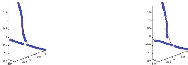
**Fig. 2.** Non-rigid registration. Intraoperative centerline points of the brain with the balloon uninflated (left) and inflated (right). The intraoperative centerline points (blue) are registered to the preoperative centerline points (red).
