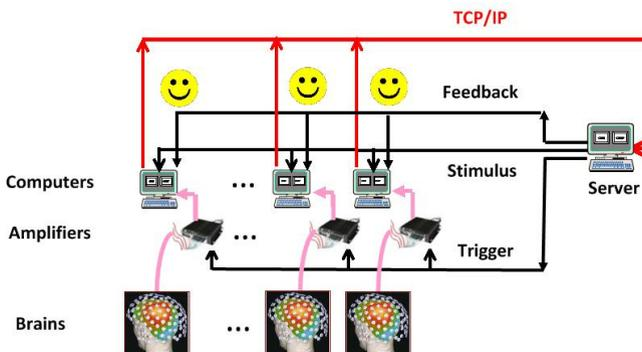
Fig. 1. Experimental setup of the collaborative BCI system
