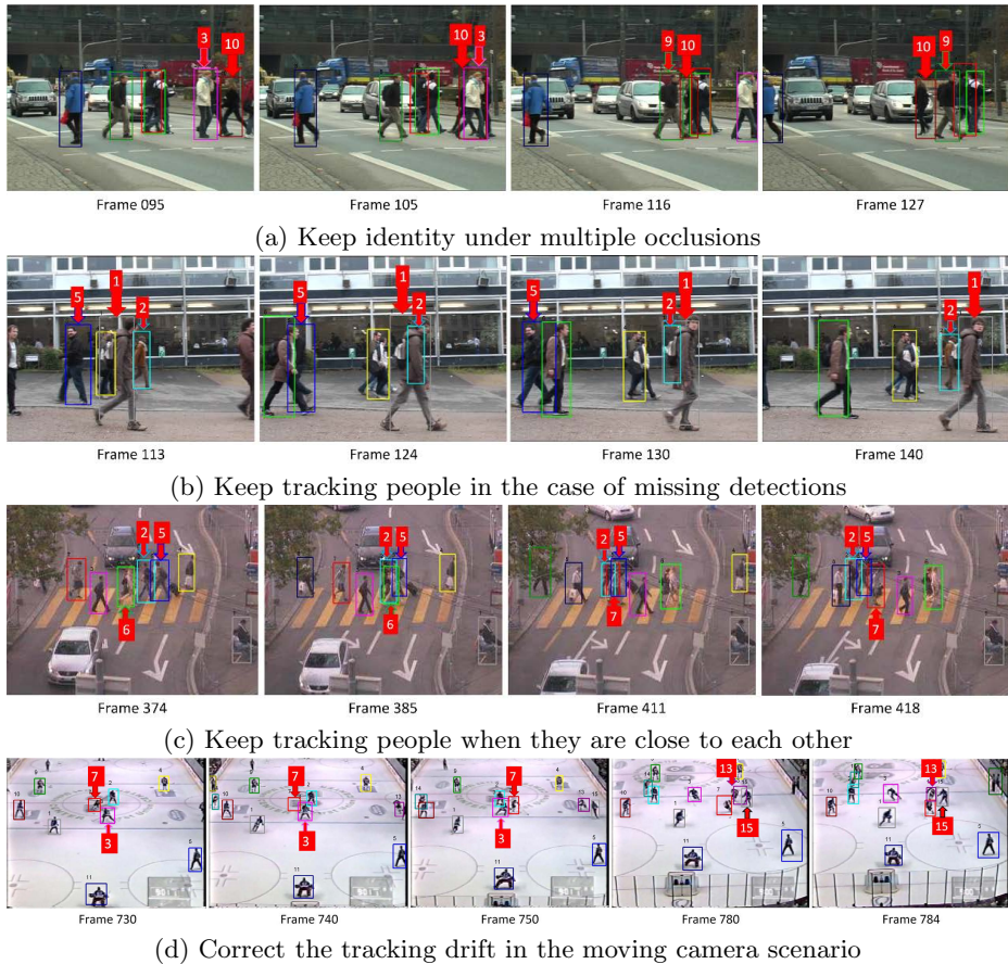
Fig. 6. Tracking results of our approach on TUD Crossing, TUD Campus, ETHZ Central and UBC Hockey datasets
