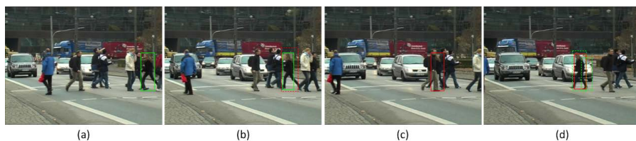
Fig. 2. Using output from both the tracker and the detector, our algorithm selects the best candidate and associates it to the tracked target. Candidates from the tracker are shown in red boxes and candidates from the detector are in green boxes. Solid boxes represent the best candidate selected by the algorithm.
