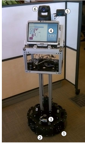
Fig. 1. CoBot-2 is equipped with 1) an omnidirectional base; 2) a 4 hour onboard battery supply; 3) a Hokuyo LIDAR sensor to detect obstacles; 4) a touch-screen tablet with wireless for onboard processing; 5) a StarGazer sensor; and 6) a pan/tilt/zoom camera
