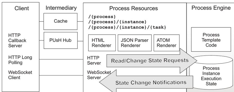
Fig. 4. Architecture of a Push-Enabled Process Execution Engine
